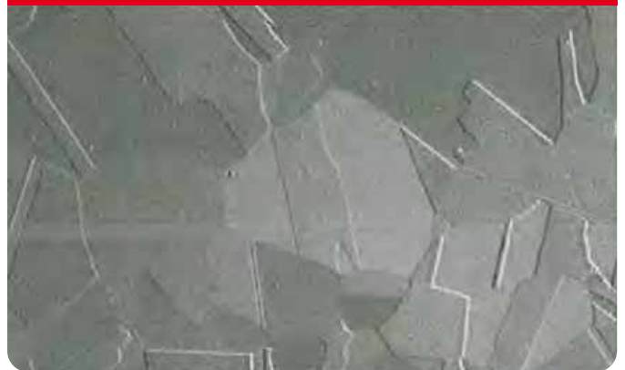
SAMPLE MATERIAL AT 100% DENSE POST- PIF (100X)
